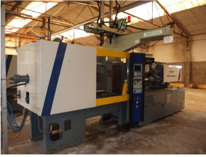
Inyectora horizontal 180 ton.Robot YMA BATTENFELD BK:T 1800/1000 Ref: 19442
